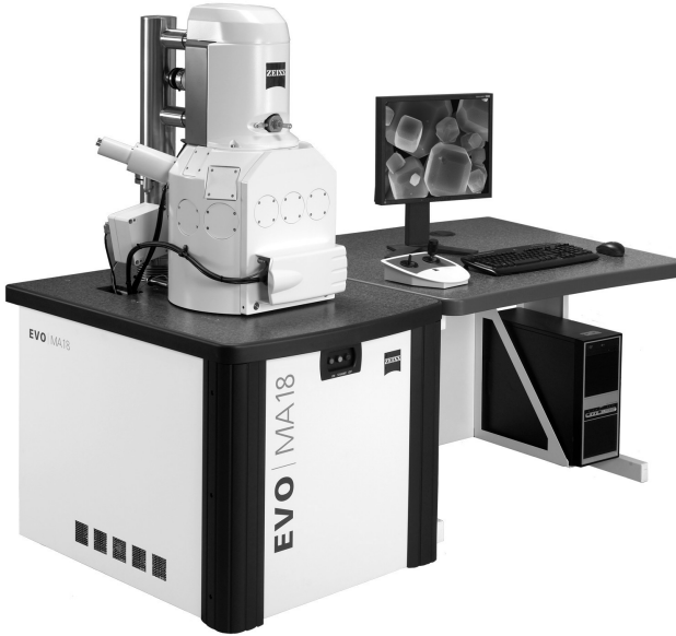
FIGURE 16.9: An SEM machine. Original image reprinted with permission from Carl Zeiss Microscopy, LLC.
